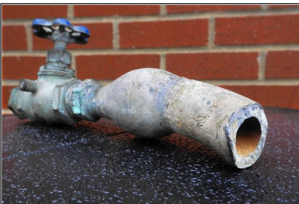
Cross section of a typical lead service line
